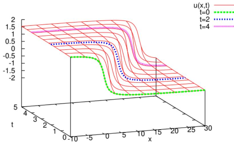
$$\frac{\partial u}{\partial t} + 5 \frac{\partial u}{\partial x} = 0, \quad u_0(x) = \arctan(-x)$$
