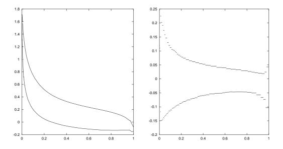
Fig. 6: Distributions of the pressure coefficient (left) and skin friction coefficient (right) along NACA0012 profile ( $M=2, \alpha=10^{\circ}, Re=500$ )
