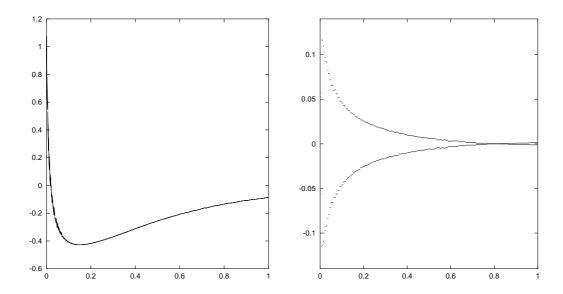
Fig. 9: Distributions of the pressure coefficient (left) and skin friction coefficient (right) along NACA0012 profile ( $M=0.5, \alpha=0^{\circ}, Re=5\,000$ )
