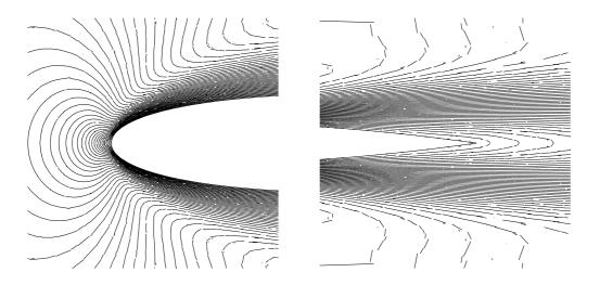
Fig. 3: Details of the Mach number isolines around the leading edge (left) and trailing edge (right) of NACA0012 profile ( $M=0.85, \alpha=0^{\circ}, Re=500$ )
