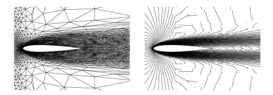
Fig. 2: Triangulation (left) and the corresponding Mach number isolines (right) around NACA0012 profile ( $M=0.85, \alpha=0^{\circ}, Re=500$ )
