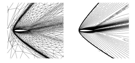
Fig. 5: Triangulation (left) and the corresponding Mach number isolines (right) around NACA0012 profile ( $M=2,~\alpha=10^{\circ},~Re=500$ )
