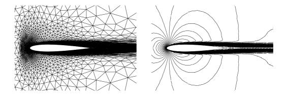
Fig. 7: Triangulation (left) and the corresponding Mach number isolines (right) around NACA0012 profile ( $M=0.5,~\alpha=0^{\circ},~Re=5\,000$ )
