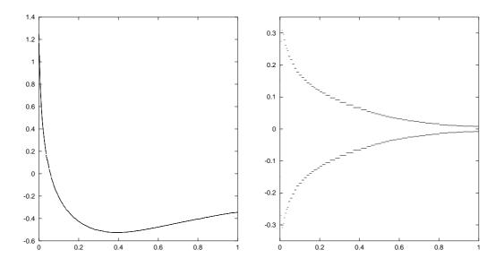
Fig. 4: Distributions of the pressure coefficient (left) and skin friction coefficient (right) along NACA0012 profile ( $M=0.85, \alpha=0^{\circ}, Re=500$ )
