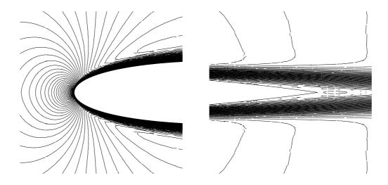
Fig. 8: Details of the Mach number isolines around the leading edge (left) and trailing edge (right) of NACA0012 profile ( $M=0.5,~\alpha=0^{\circ},~Re=5\,000$ )
