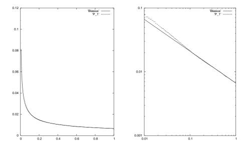
Fig. 1: Distribution of the computed skin friction coefficient (P<sub>-</sub>1) with the "theoretical" one (Blasius). The left and right figures are plotted in linear and logarithmic scaling, respectively
