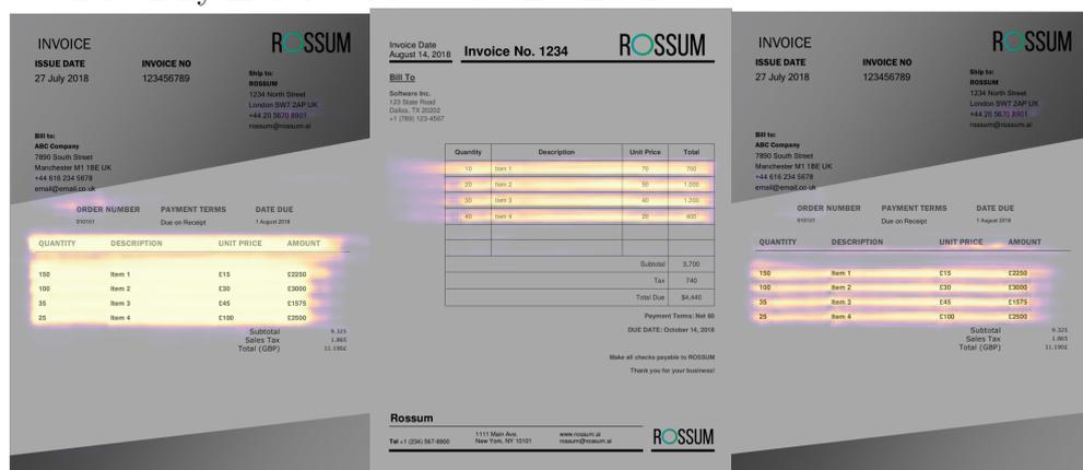
In parallel, we also work on hybrid methods (a combination of the older methods mentioned above and artificial intelligence). Here are some examples of column search, based on custom image-processing features and learned 1D dilated segmentation.
