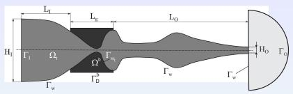
Geometry of the computational domain at time t=0 and the description of its size:  $L_I=20.0$  mm,  $L_g=17.5$  mm,  $L_O=55.0$  mm,  $H_I=25.5$  mm,  $H_O=2.76$  mm.
