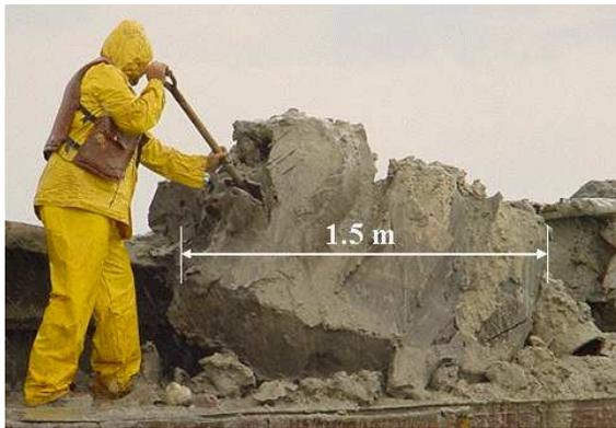
FIGURE 3. Clay lump of Singapore marine clay dredged from the seabed
