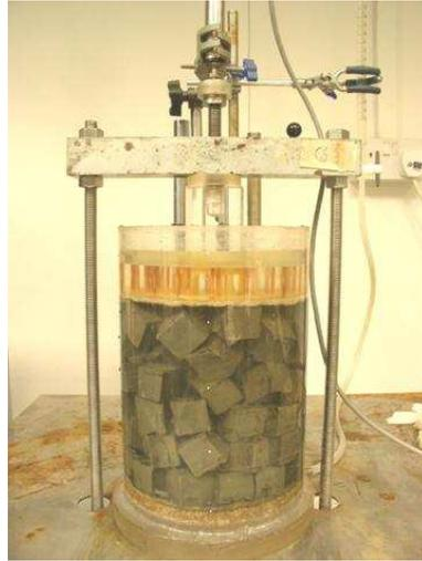
FIGURE 4. Experimental set-up for the lumpy fill experiments
