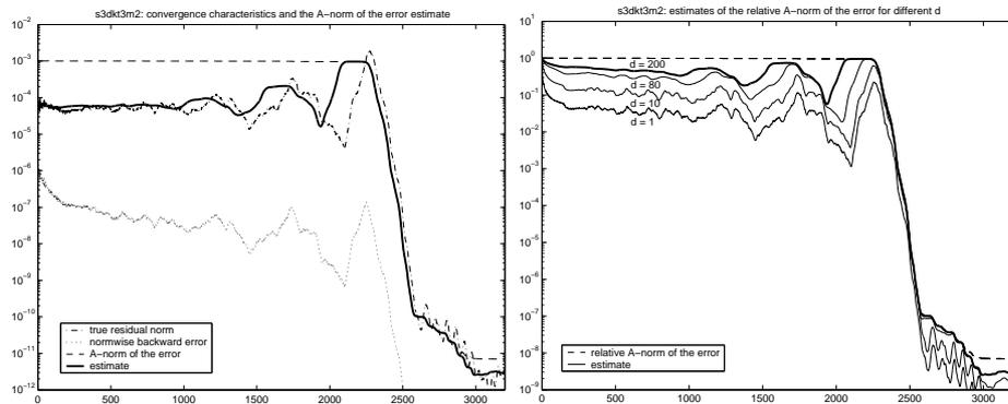
Figure 5.1: The system `s3dkt3m2`. In an extremal case of very slow PCG convergence the estimate  $\nu_{j,d}^{1/2}$  can significantly underestimate the actual  $A$ -norm of the error (left part). The estimate  $\varrho_{j,d}^{1/2}$  of the relative  $A$ -norm of the error (right part) is in general much tighter than the estimate of the  $A$ -norm of the error.
