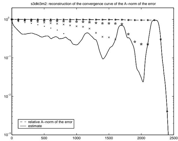
Figure 5.4: The system `s3dkt3m2`. The relative  $A$ -norm of the error (dashed line), the estimate of the relative  $A$ -norm of the error with  $d = 100$  (solid line) and the curves reconstructed at iterations 1000 (dots), 1700 (x-marks), 2200 (pentagrams) and 2500 (stars).
