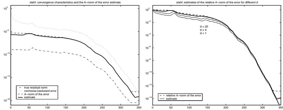
Figure 5.3: The system `stahl`. The estimates for the absolute and relative  $A$ -norm of the error are tight throughout the whole computation.
