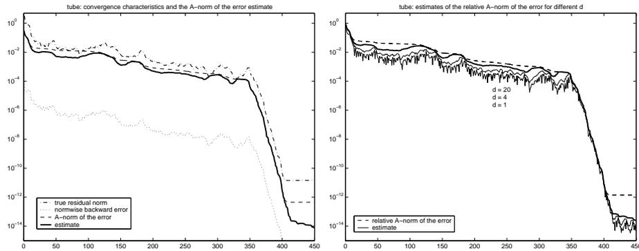
Figure 5.2: The system `tube`. Even a slow decrease of the  $A$ -norm of the error is sufficient for obtaining a satisfactory value of the estimate  $\nu_{j,d}^{1/2}$  of the  $A$ -norm of the error. The erratic behaviour for  $d = 1$  is caused by the oscillations of the coefficients  $\gamma_j$  (right part). By increasing the value of  $d$ , the curves are more smooth and closer to the relative  $A$ -norm of the error.
