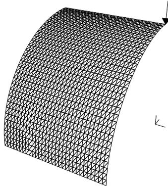
In our experiments we use the matrix `s3dkt3m2` of the order  $n = 90449$ . The matrix has  $\text{nnz}(A) = 1921955$  nonzero elements, and the condition number  $\kappa(A) = 3.62e+11$ . Only the last element of the right-hand side vector  $b$  is nonzero, which corresponds to the given physical problem (for more details see [24] and the references in [24]). The preconditioner was determined by incomplete Cholesky decomposition with no fill-in.
