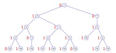
Seems to use TIME(N) and SPACE(N). But space can be re-used. In this example, 3 memory bits suffice.
