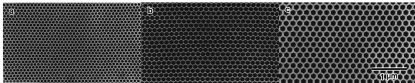
FIG. 5. SEM micrographs of cell configuration in barrier layer with different intervals of 100 nm (a), 150 nm (b), and 200 nm (c). Anodization voltage were 40 V (a), 60 V (b), and 80 V (c). Anodization was conducted in 0.3 M oxalic acid of 17 °C for (a) and (b), and 0.04 M oxalic acid of 3 °C for (c). Thickness of the oxide films was approximately 3 μm.
