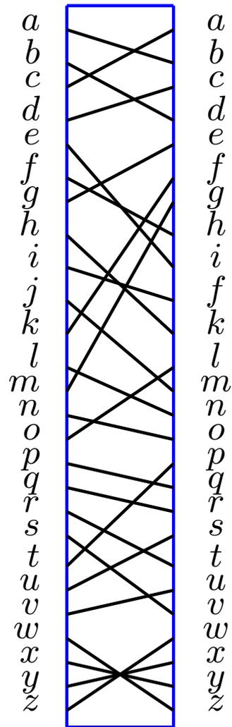
If we take a rotor, we may denote the spring contacts on one side of the rotor by the letters of the alphabet  $a, b, c, \dots, x, y, z$ . Opposite to each spring contact there is a disc, through which the current flows out of the rotor. We denote it by the same letter as the opposite spring contact. Thus the wires inside the rotor define a permutation on the alphabet  $\{a, b, c, \dots, x, y, z\}$ .
