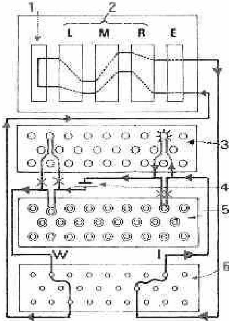
This is how the current flows through the Enigma machine after pressing a key.
